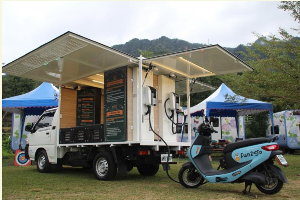
Mobile 24kW EV DC fast charger (15kW mGen) fuel: 100L (~100kWh)
